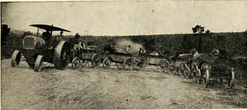
These six wagons are less than half a load for this Twin City "25" used by the Taxpayers' Association of Hazelton, Penn.
